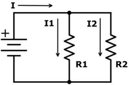
Figure 4. A parallel circuit.
