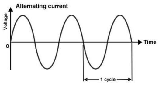
Figure 2. An alternating current (AC) waveform.
