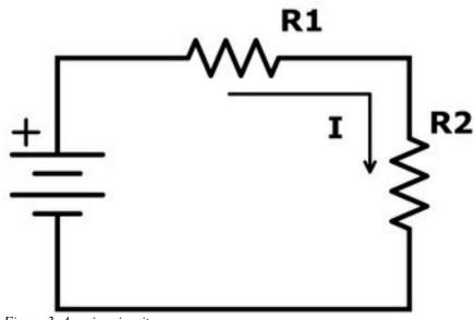
Figure 3. A series circuit.
