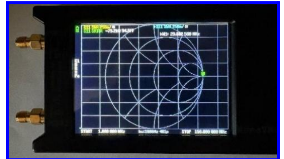
Fig 1: NanoVNA H4 Showing 'Port Savers'
