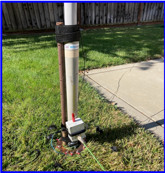
Figure 1: Base of the antenna showing the mast, radial connections, and matchbox.
